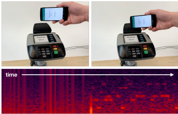
Figure 1: VibroComm uses the gyroscope sensor found in phones for vibroacoustic data communication. Objects hovering above surfaces receive no data (left). Only when physical contact is made is data received (right). This makes interactions targeted and explicit, requiring presence and intent.
