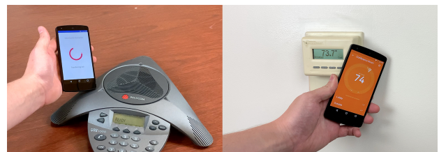
Figure 10: Left: VibroComm could be used to handoff functionality from one device to another, as seen with this conference room speaker. Right: Full-featured apps could be automatically launched in response to a user touching their phone to a smart device, for example, smart thermostats.
