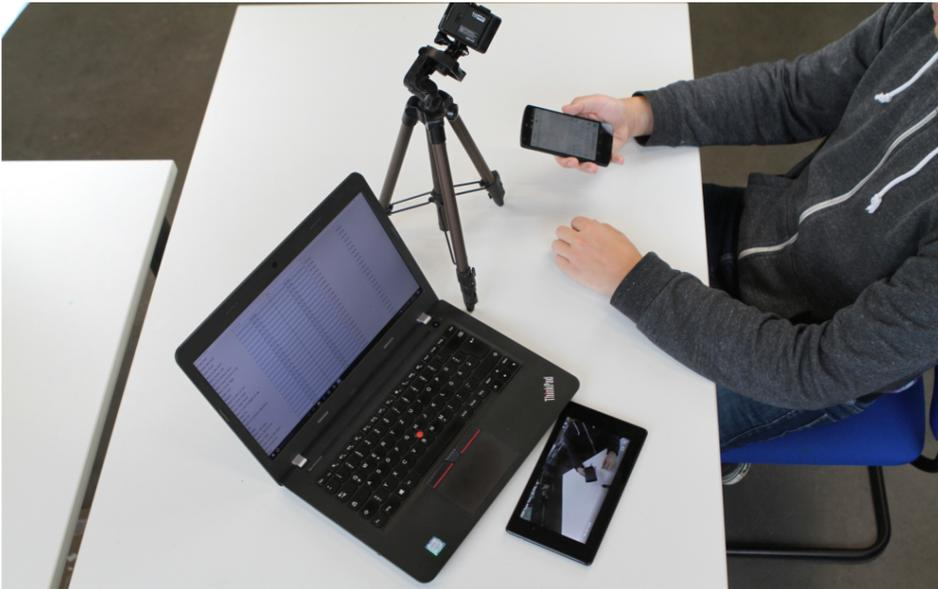
Fig. 2. Setup for the elicitation study. We used the tablet for camera preview and the laptop to control the referents on the smartphone.
