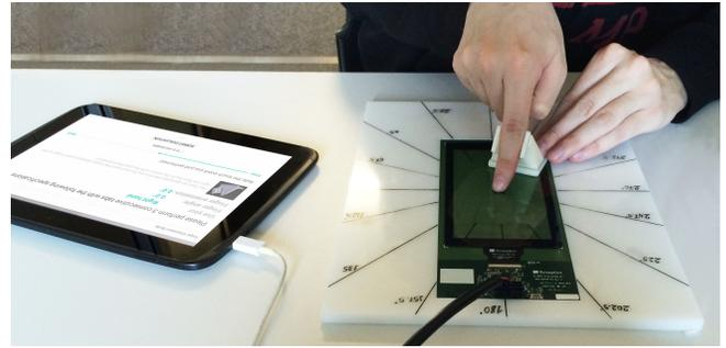
**Figure 4.** The apparatus we used in our study, showing the tablet, the touch layer and one of the pitch stabilizer while one participant touches the touch surface.
