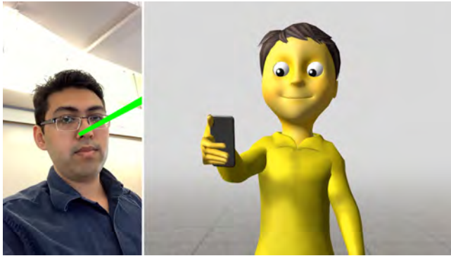
Figure 2: Left: User-facing camera view with head vector shown in green. Right: Avatar with corresponding head pose. Note that eye gaze is also captured and applied to the avatar.
