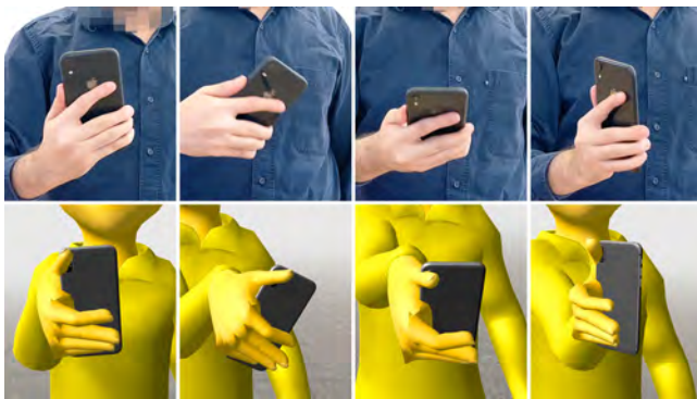
Figure 5: Phone orientation (pitch, yaw, and roll) is used to control the phone prop and better pose the wrist and hand.
