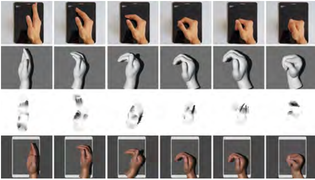
Figure 6: Six snapshots showing a hand transitioning from an chop (pose M) to a fist (pose P). First row: reference photos. Second row: closest reference pose. Third row: displacement field between the live input and best pose. Bottom row: final 3D hand output pose.
