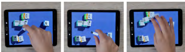
Figure 12: In this BumpTop-inspired demo [2], users can pick up files (left & center), create piles, and push documents around (right).
