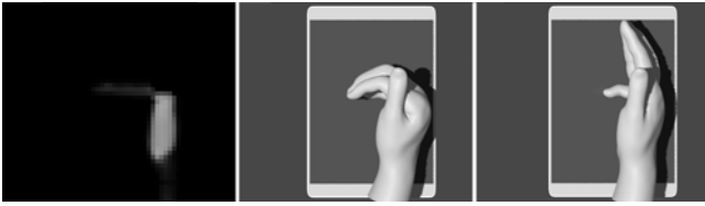
Figure 8: Example of additional pose logic. Although only the pinky is captured in the touchscreen capacitive image (left), we decide to animate all of the fingers as one unit (center), as opposed to just moving the pinky alone (right), as this is less natural.
