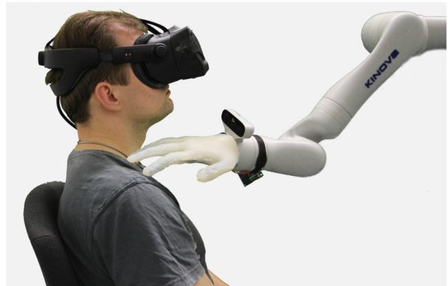
Figure 1: The Social Touch example; we used Cobity to deliver human like touch sensations in virtual reality.
