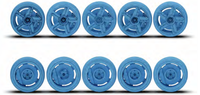
(b) Original (far left) and 4 reduction variants, all rated as 5 in the same iteration. The bottom row shows the backside of the models. Objectively, the middle left wheel contains faulty geometry and should receive a 0 ( skip ) rather than a 5 ( excellent ).
