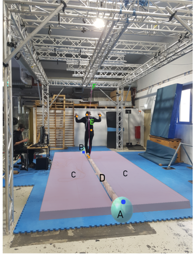
Figure 3: Study apparatus with trigger zones overlay. A: Start Zone, B: End Zone, C: Fall Zones, D: Step Zone; E: Safety Harness, F: Rope Slide; Orange dots: 6 on-body position trackers (head, hands, feet, waist), blue dots: 2 beam position trackers used for scene matching. Each trigger zone was activated or deactivated by one of the feet trackers entering or leaving it.
