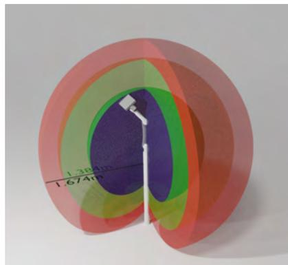
Fig. 5. Rendering reachable volumes: nominal space of the robot  $3.29m^3$  (Blue), space within ideal rendering quality  $7.42 m^3$  (Green) and maximum rendering space  $8.27m^3$  (lower quality, in Red). This is  $19.98 m^3$  Volume in total.
