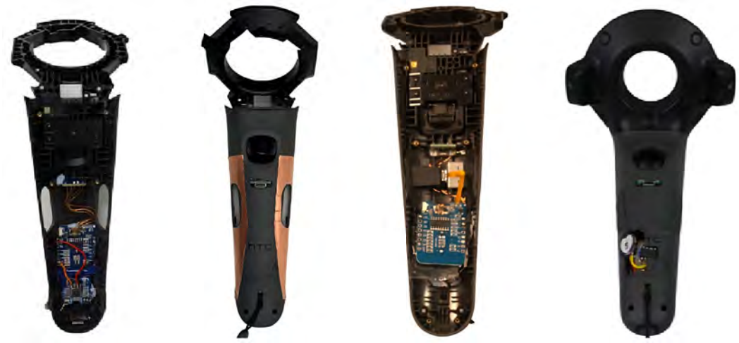
Fig. 3. EDA and PPG sensors integrated into VR controllers. In the first picture, EDA sensor is integrated into a controller. In the second figure, two copper stripes measure the EDA when a user picks up the controller. In the third figure, PPG sensor integrated inside the controller. In the fourth figure, the PPG sensor measures the user's HR by implicitly pressing the palm against the sensor.
