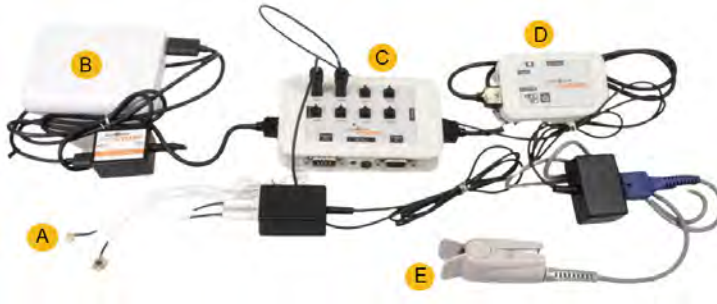
Fig. 5. The medical-grade system used as gold standards for evaluating SensCon-based EDA and PPG measurements. The EDA electrodes (A) and PPG finger clip sensor (E) are connected to the AUX ports of the Sensor & Trigger extension (STE) (C). For signal amplification and streaming to the acquisition PC, we use a LiveAmp amplifier (D) and a power bank for energy supply to the STE (B). All components were placed inside a pouch and comfortably worn by participants across the experimental sessions
