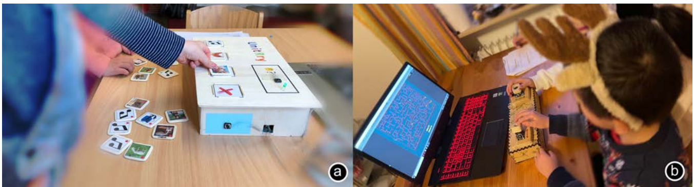
Figure 1: The tangible prototypes UnitRry and CollabMaze we developed and evaluated. a) Two children put knowledge cards on UnitRry to learn relations of chicken, egg, and chicken cluck. b) One child controls left-right, the other controls up-down of the CollabMaze to move the character out of the maze.
