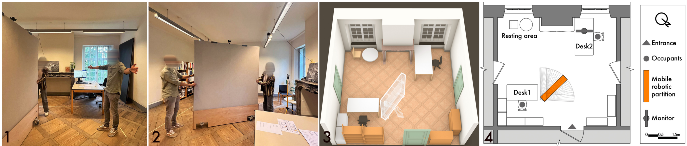
Fig. 1. During improvisation sessions, 15 experts designed gestures for a mobile robotic partition by first bodystorming how to convey an intent (1), then manually manoeuvring the partition with a researcher to perform the accordant gesture (2), before reviewing the 3D visualisation of the gesture as recorded via a real-time motion-capture system (3), and comparing all designed gestures in a questionnaire while viewing their 2D animations (4) side-by-side.
