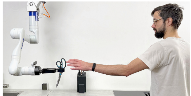
Figure 1: We investigate the preferred speed and distance when handing over objects varying in perceived danger.
